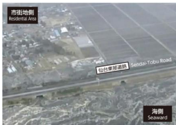
The Sendai-Tobu Road blocked the tsunami and rubble from reaching farther inland
