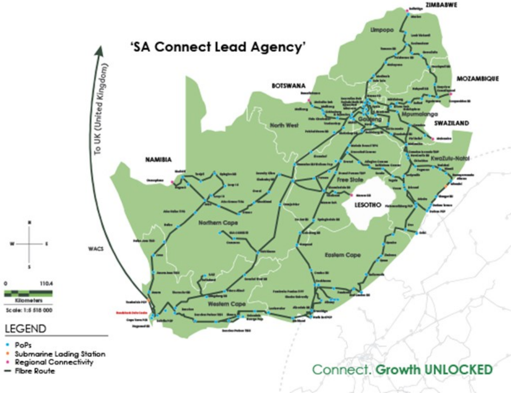
Figure 3.6.1 Situation of the Domestic Backbone Network
