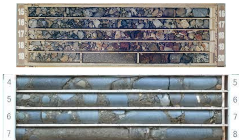
Figure 17.3-1 Comparison Core of Conventional Method (upper) and Advanced High Quality Boring Method (lower)
