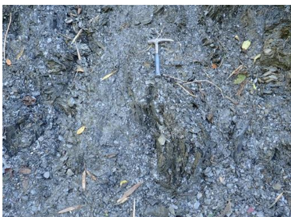
Figure 13.2-6 Highly fractured carbonaceous phyllite
