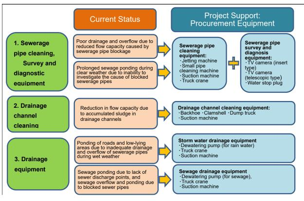
for sewer pipe survey is needed with a view to change the sewer pipe management method.
