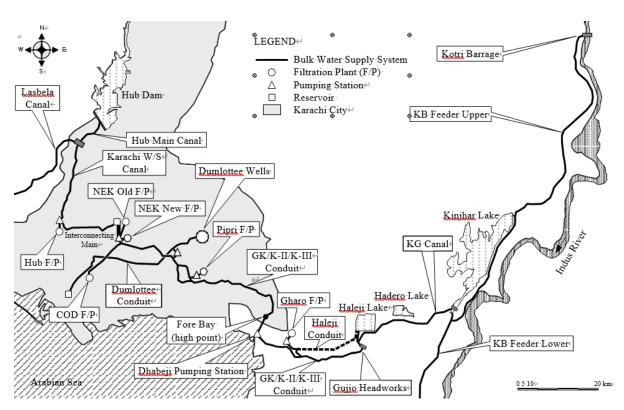
Figure 5.5-3 Bulk Water Supply System in Karachi City
