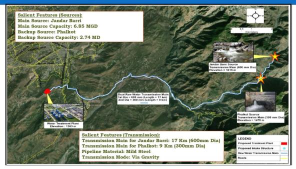
Source : ADB, CEC Minconsult, KPCIP-04: Extension of JICA Gravity Water Supply Scheme Detailed Engineering Design Figure 4.9-1 Layout of Water Intake Facilities, Low Water Pipeline and Water Treatment Plants
