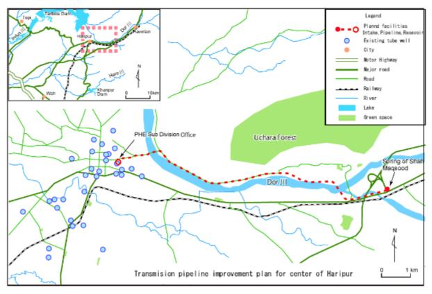
Figure 4.8-1Existing Tube Well Layout and Planned Transmission Pipeline Route for the Urban Water Supply System
