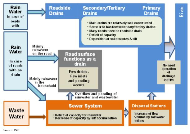
Figure 6.4-2 Sewage and Rainwater Drainage System in Lahore
