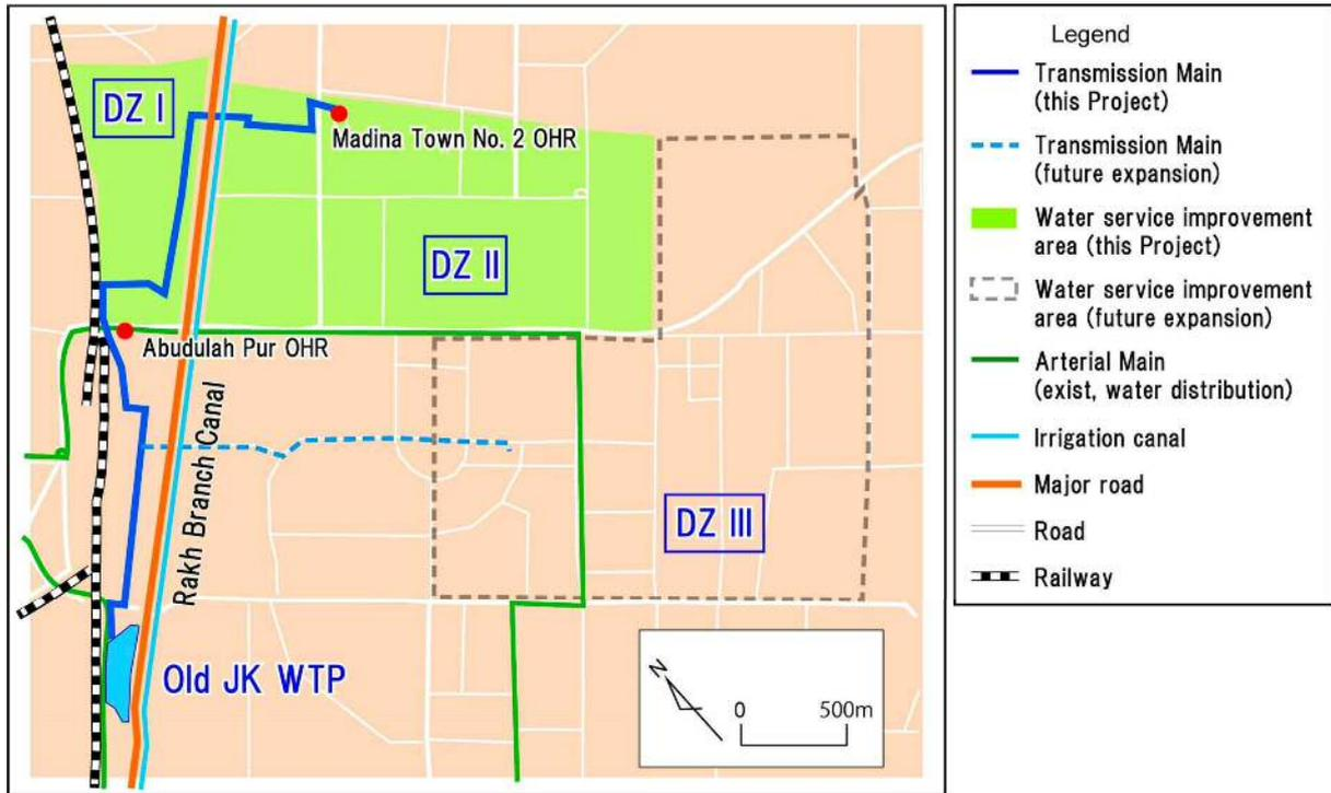
Fig. 3 Water Service Improvement Area for Outline Design in Preparatory Survey
