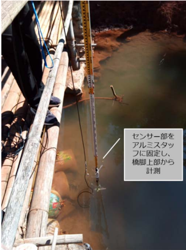
Fig10 Measuring water velocity in the field
