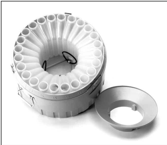
Fig-18 Sample container bottle stored inside of ISCO
