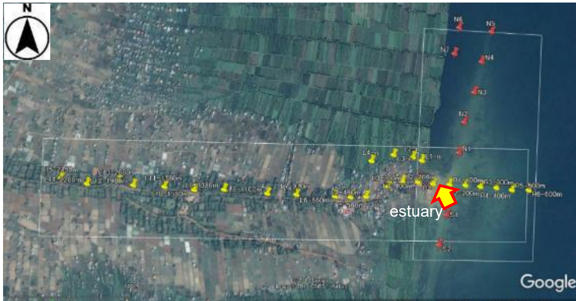
Figure 5. Target area and surface water sampling locations (34 locations)* Red pin indicates additional points
