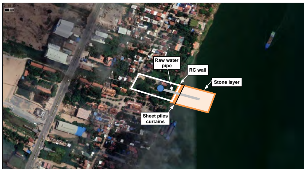
Figure 6.2.11 Outline Plan of Proposed Protection Of Revetment and Riverbed for Bakheng Phase III
