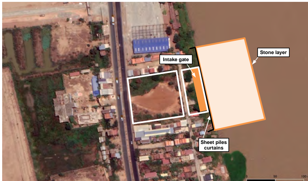
Figure 6.2.17 Outline Plan of Proposed Protection of Revetment and Riverbed for Ta Mouk Source: JICA Data Collection Survey Team
