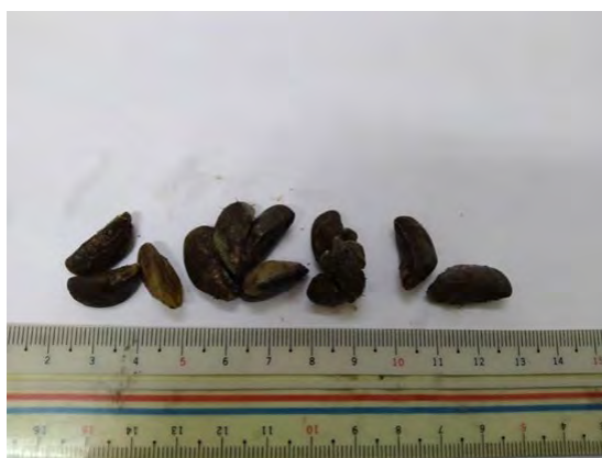
Figure 6.2.19 Shellfish attached inside the chamber of intake tower
