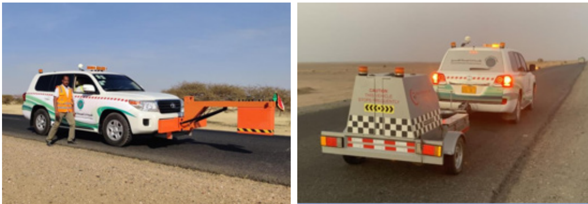
Figure 2-4-11 Field Survey Using GPR (left), Field Survey Using FWD (right)
