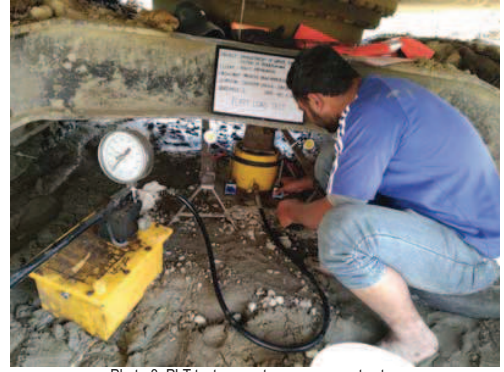
Photo-3: PLT test apparatus arrangement setup
