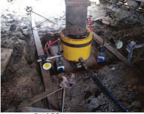
Photo-3: PLT test apparatus arrangement
