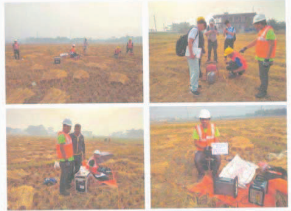
Cable Layout and Data acquisition of VES-1 (NWSC -7)
