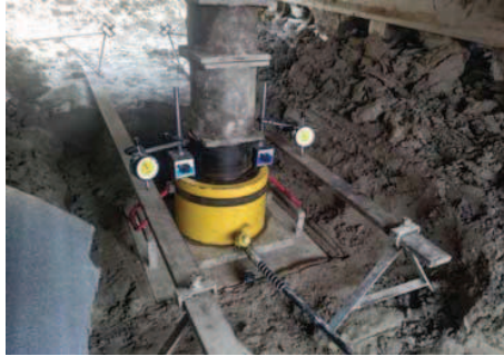
Photo-3: PLT test apparatus arrangement
