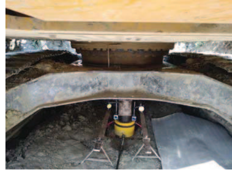
Photo-3: PLT test apparatus arrangement
