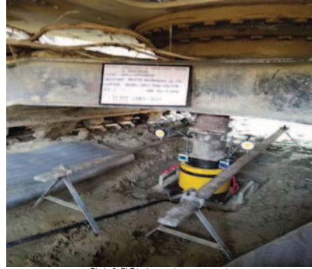
Photo-3: PLT test apparatus arrangement
