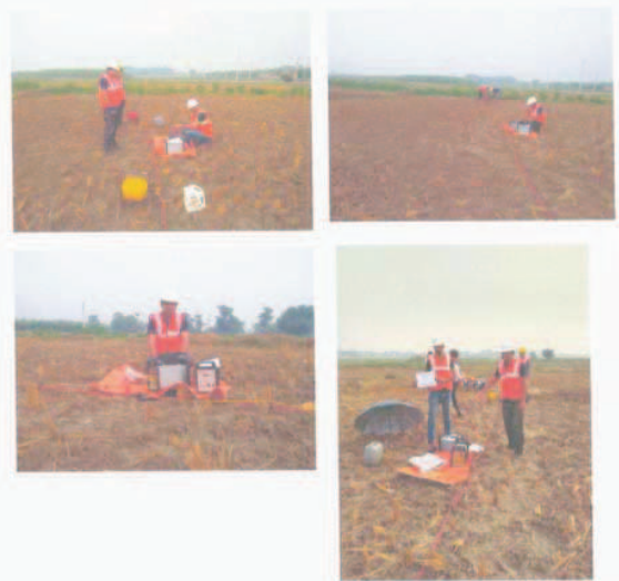
Cable Layout and Data acquisition of VES-5 (NWSC- 5)
