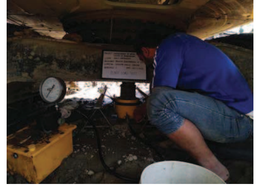
Photo-4: PLT test apparatus arrangement setup
