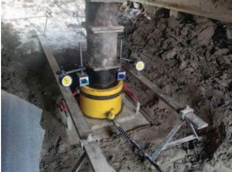
Photo-2: PLT test apparatus arrangement
