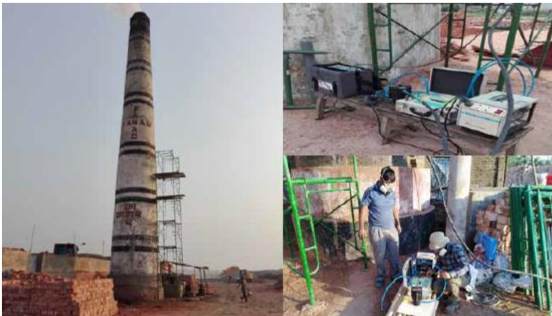
Figure 5.1-21 Sampling of exhaust gas from a brick kiln in the CASE project
