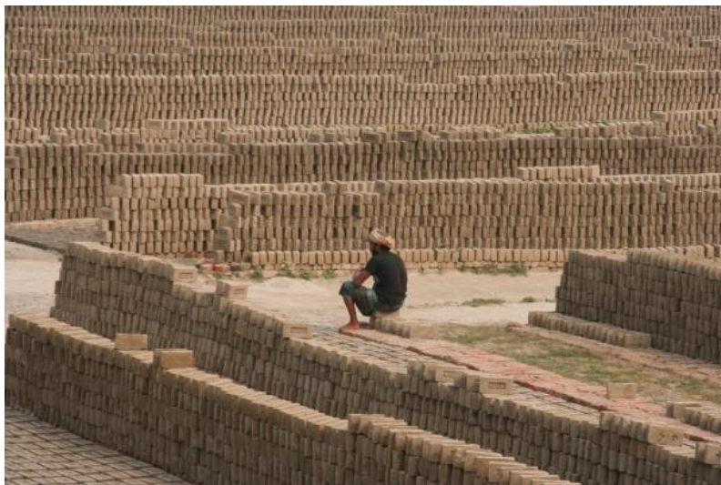
Figure 5.1-19 Bricks before burning being dried in the sun
