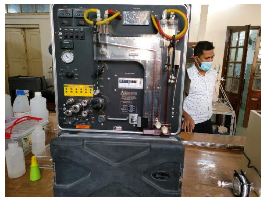
Figure 5.1-5 Equipment for stationary source emissions investigation owned by BUET Chemical Engineering Department
