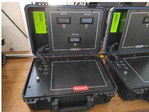
Figure 5.1-5 Equipment for stationary source emissions investigation owned by BUET Chemical Engineering Department
