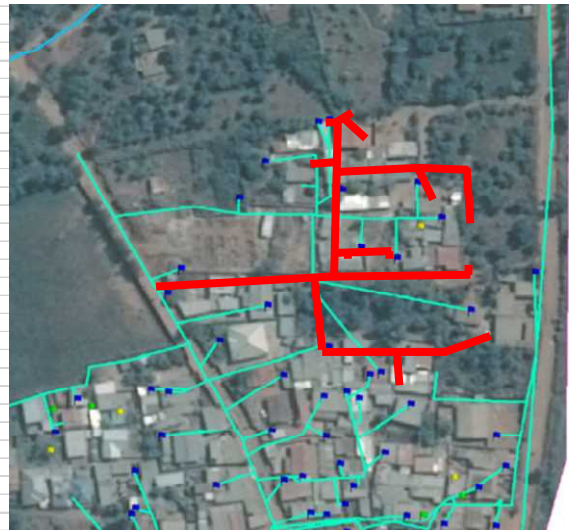
Figure 2.7.3 Pipe routes on GIS map (green) and those confirmed on site (red)
