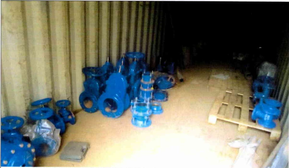
**FLOAT VALVES AND VALVES AT KIMISAGARA WTP, BEFORE INSTALLATION**
