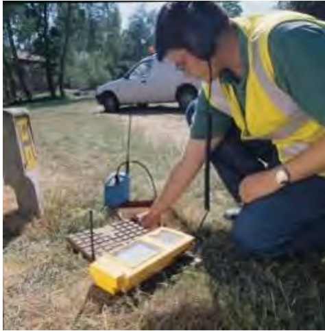
An „advanced“ leak noise correlator, showing the correlation peak.
