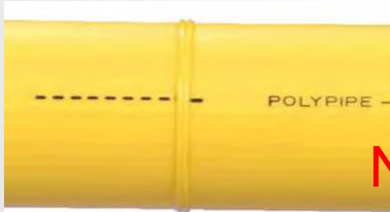
Melt bead too small due to insufficient heat time
