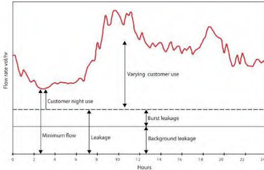
FIGURE 7.2: TYPICAL 24-HOUR DMA FLOW PROFILE
