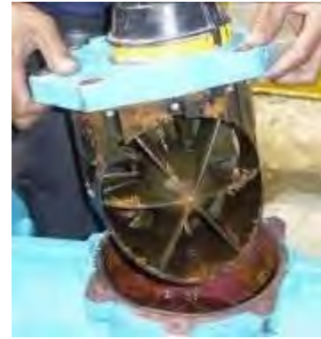
Sedimentation is a major cause of meter reading inaccuracies.
