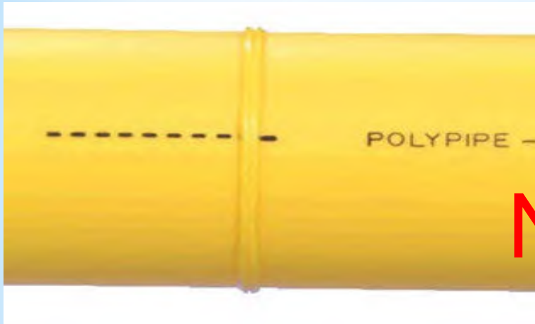
Melt bead too small due to insufficient heat time
