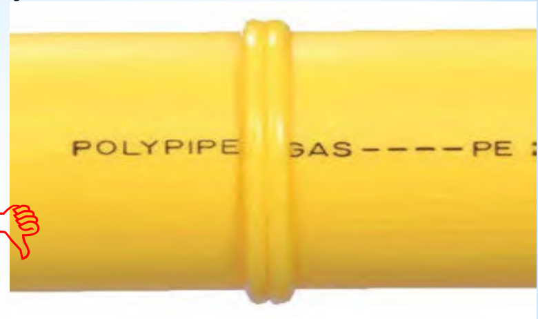
Melt bead too large due to excessive heating and/or over pressurization of joint
