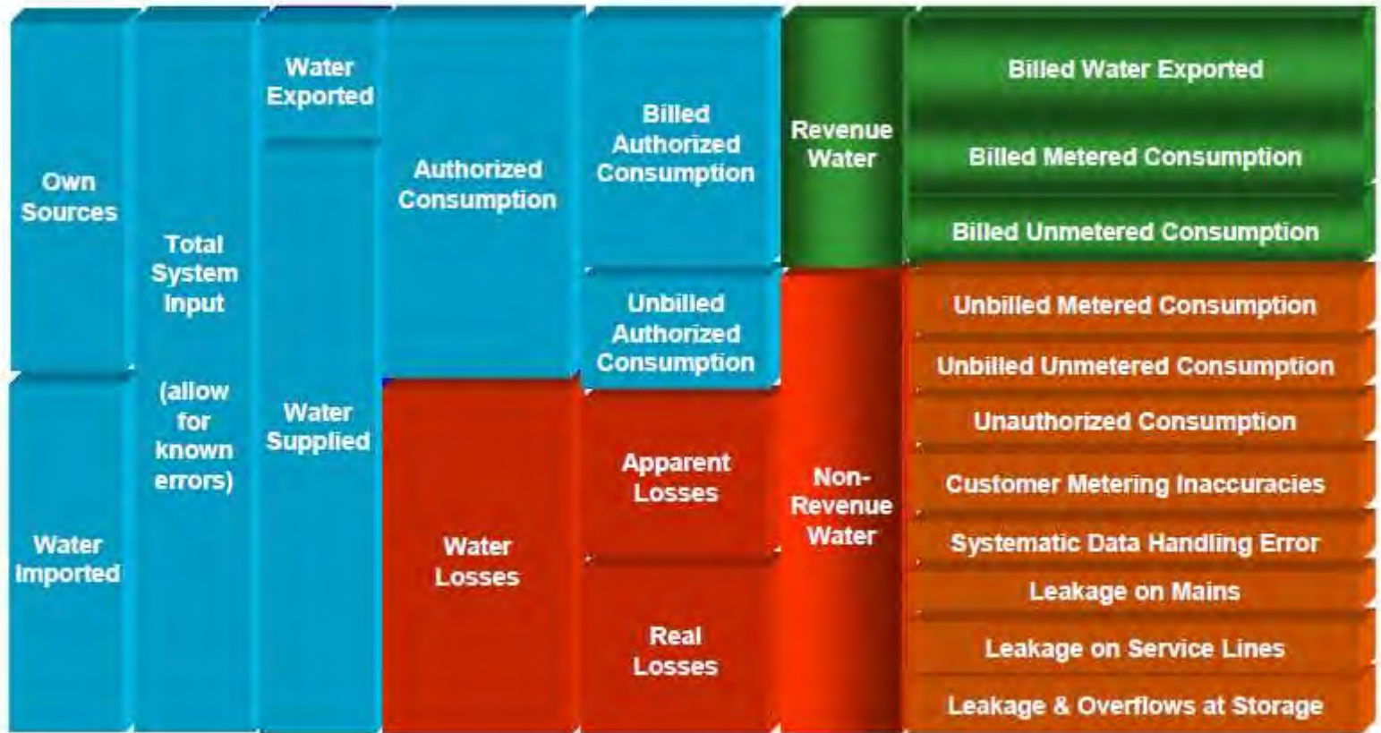
Figure 1 the AWWA/IWA Water Balance Table
