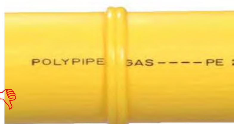
Melt bead too large due to excessive heating and/or over pressurization of joint
