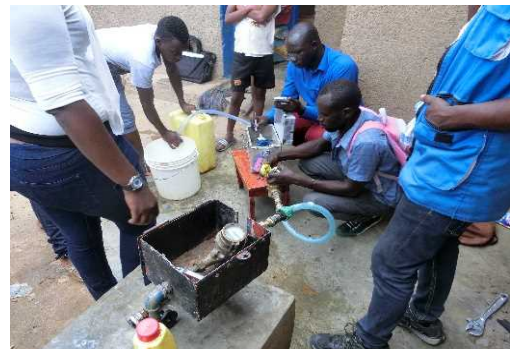
On-site Meter Accuracy Test
