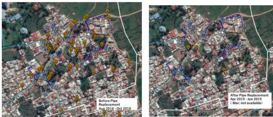
Fig. 1 Plotting of the Leakage Repair Point
