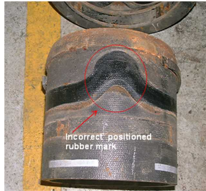
Fig.14 Leaks caused by incorrect positioned rubber ring
