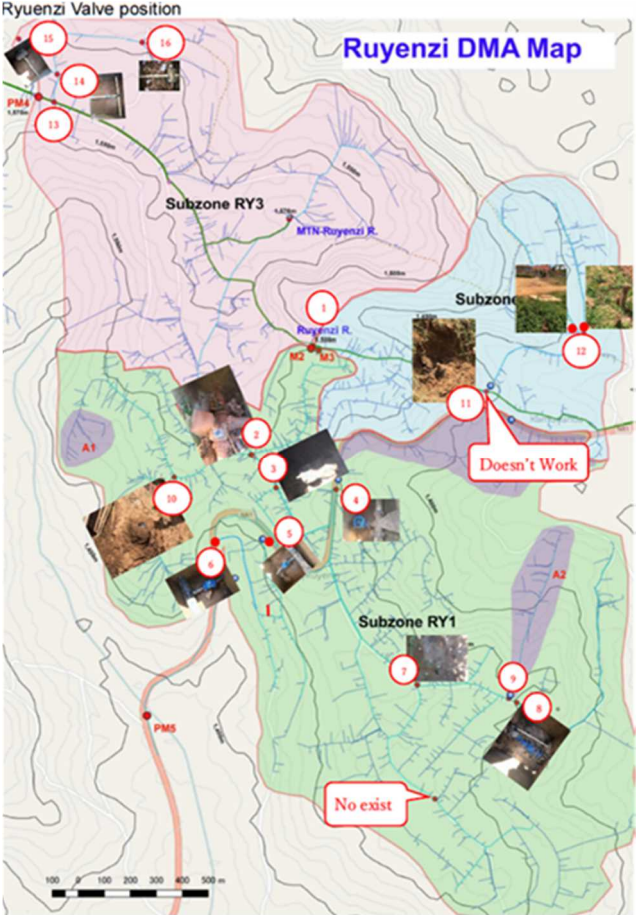
Figure 2.4.2. Locations and working status of gate valves
