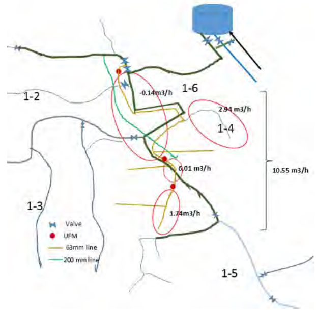
Figure 31. Measurement of flow rate in 63-mm distribution pipe, Step Test, June 20, 2019
