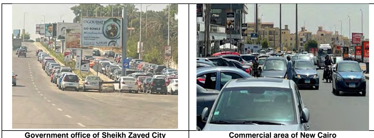
Figure 3.3.7 Road capacity reduction due on-street parking
