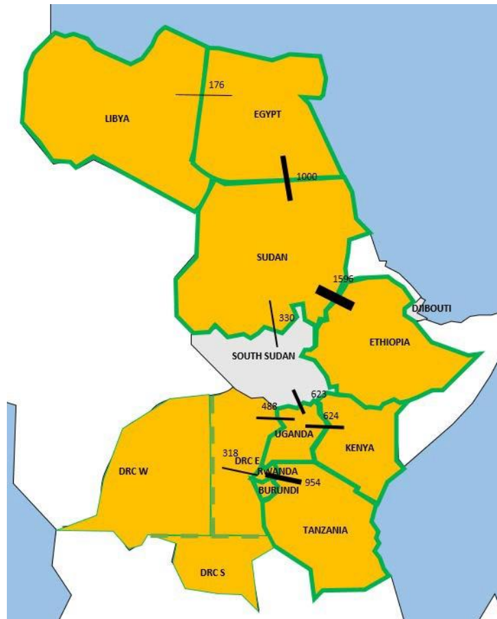
出所 Figure 22. Recommended new lines by 2025. Numbers indicate capacity in MW、EAPP Regional Power System Master Plan、2014
