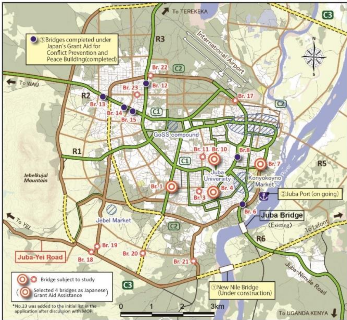
Figure 2-2-2 Result of Selection of the Surveyed Bridge
