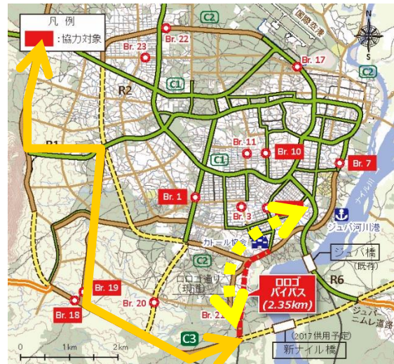
Step-1: Formation of Ring Road and connection to the river port and city central and Nimule road by Lologo bypass
