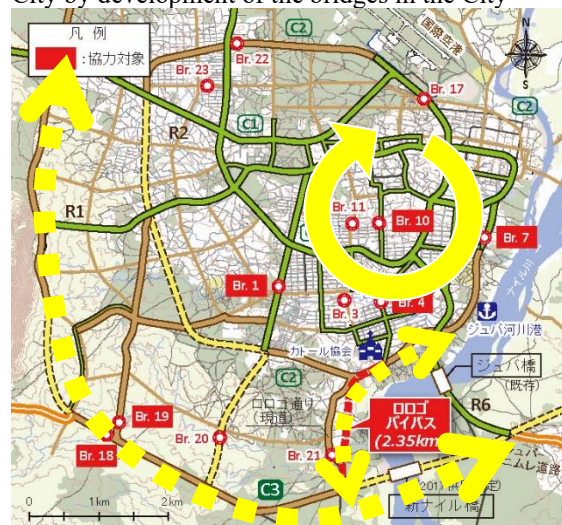
Step-3: Development of international logistics road by erection of bridges located on Ring Road C3
