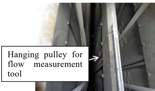
Velocity measuring instrument hanging tool Operation check at ESP lower floor
