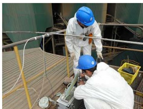
Pictures of the exhaust gas measurement at TPP Kosovo A
