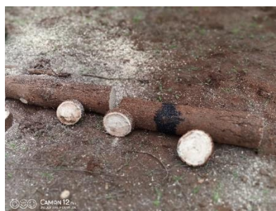
Plate 10. Wood discs collected at three trees height level
