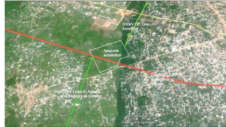
Figure 2.6 Dense Residential Area Around Ajegunle Substation
