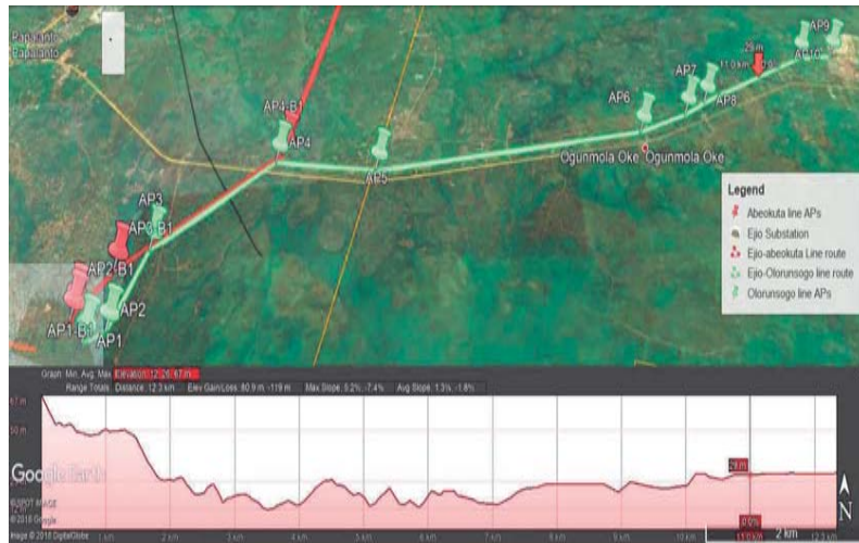
Figure 2.3 Ejo to Olorunsogo Line showing line route
