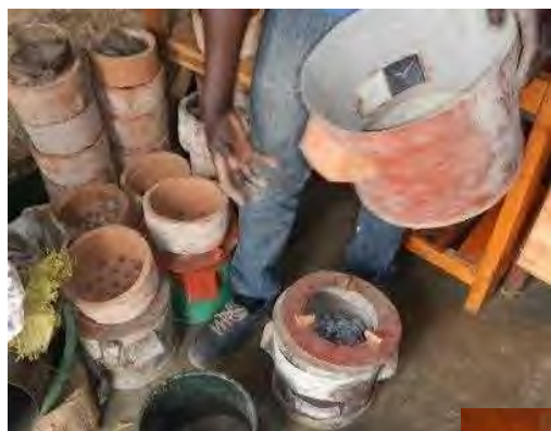
stove for briquettes/charcoal with a clay liner (Nebbi)
