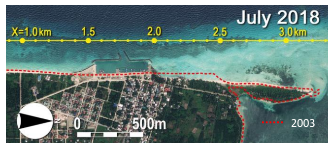
Figure 26 Coastal Change after Port Construction (Gan Island, Red Line: Shoreline as of 2003)
