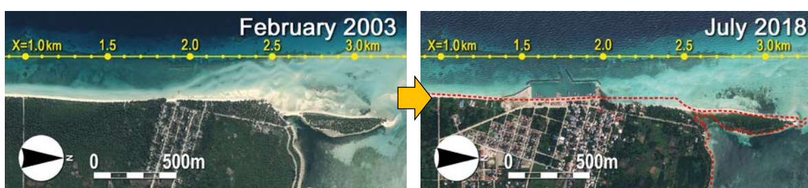
(1) Coastal Erosion due to Harbor Construction (Gan in Laamu Atoll)
