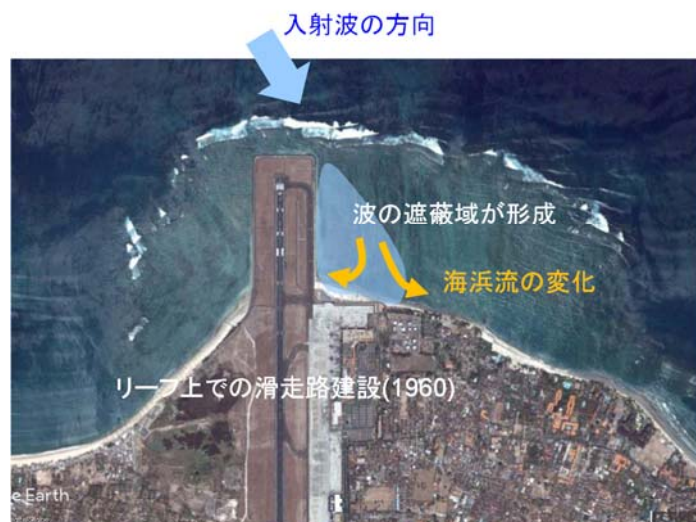
Figure 1.4.5 Longshore Change in Shoreline since 1960 (Source: Syamsudin (1993), "Beach Erosion in Coral Reef Beaches and Its Control")
