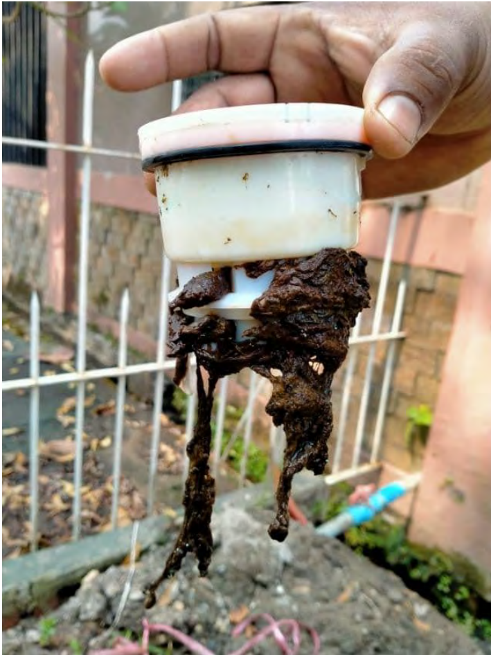
Clogging water meter with impurities
