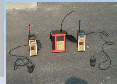
- Correlative Leak Detection Equipment
