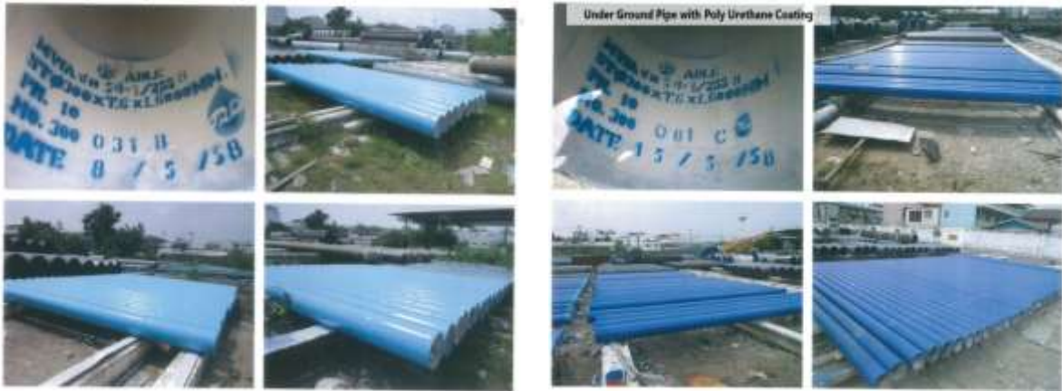
External Coating by AWWA Standard Jointing of underground pipe
