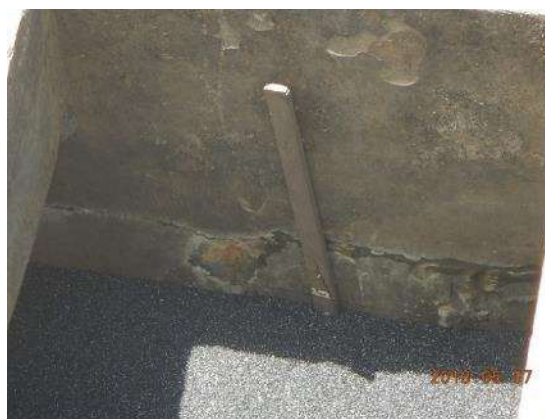
Replaced anthracite (Phase 1 pilot filter)
