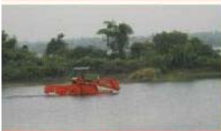
Removal of weeds by Aquamarine to clean
