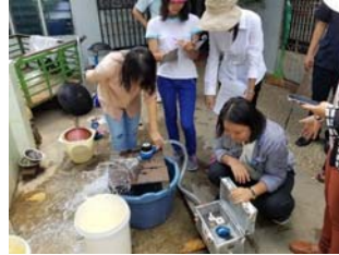
Meter function test by test meter
