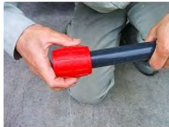
2- Scraping the outer circumference
