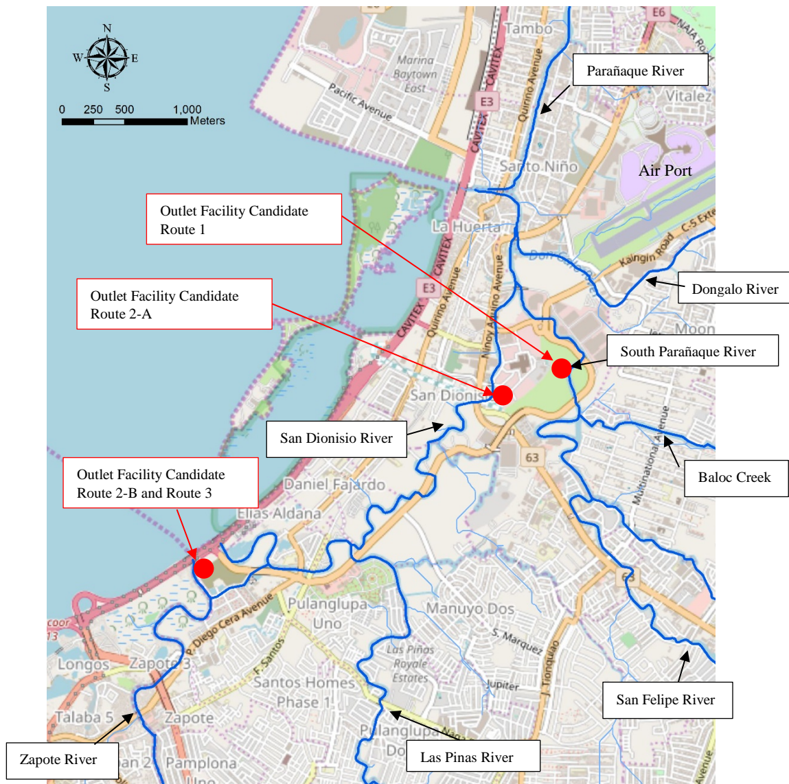
Figure 4.7.1 River Network System in Las-Piñas and Parañaque
