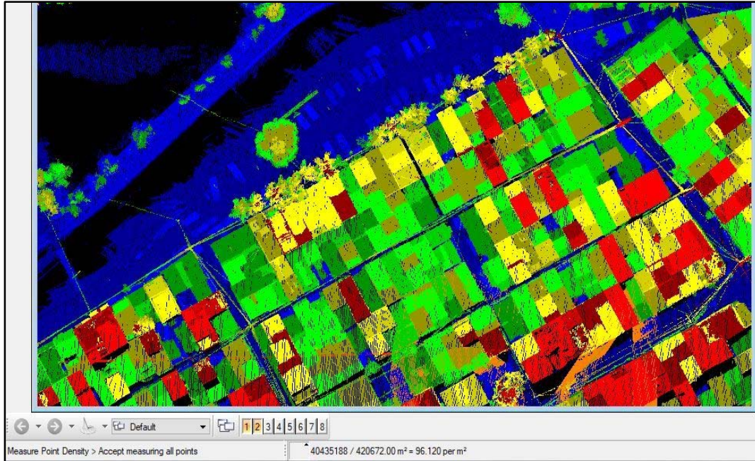
Figure 16 LiDAR pointcloud density per m 2
