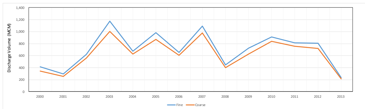
Figure 5.5.13 Discharge Volume Trend with Threshold Snowmelt Temperature during Snowmelt Season (March-June)
