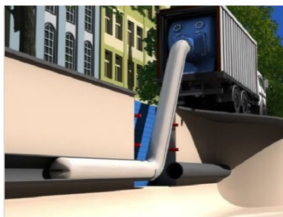
CIPP (Cured In Place Pipe) арга
