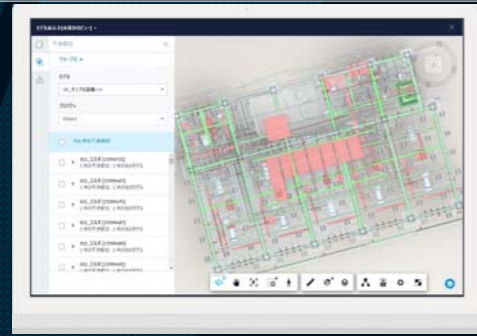
Check the crash position from BIM 360 Coordinate
