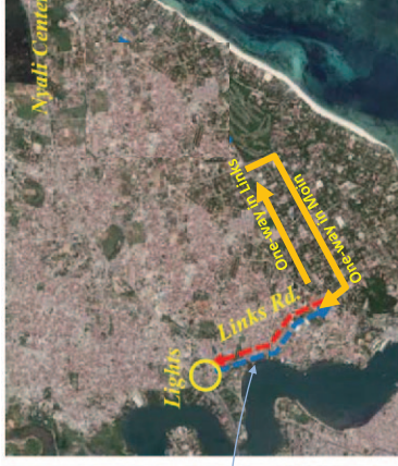
Image of the reversible lane operation and signal installation in Links Rd three-lanes section
