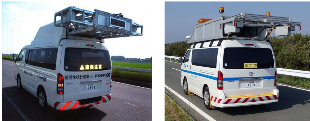
Figure 5.5.9 Road Surface Texture Measurement Vehicle
