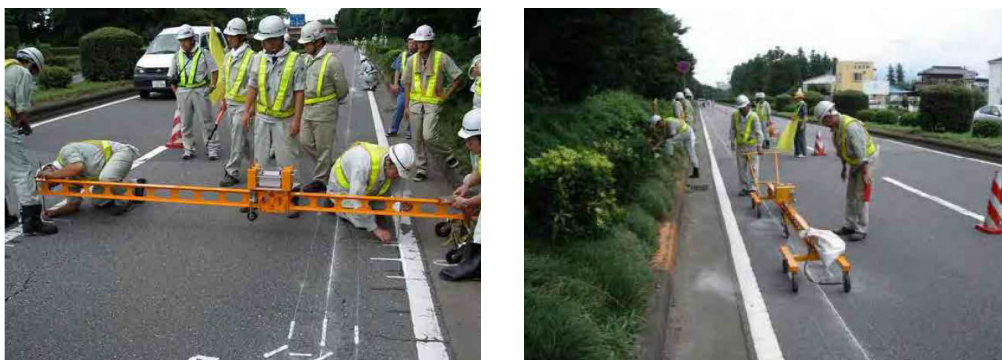
Figure 5.5.8 Measurement by Using Profile Meter
