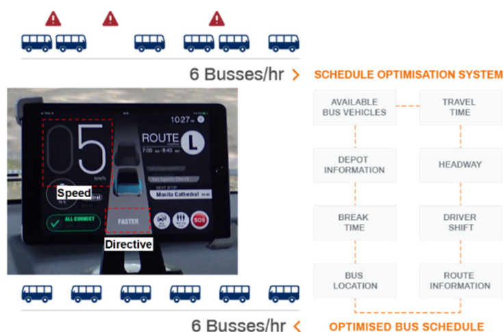
Figure 5.3.10 Image of an Interval Management System for Public Transportation
