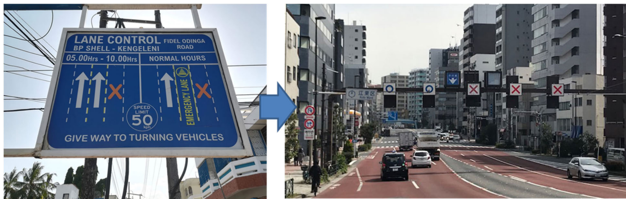
Figure 6.3.7 A Sample of Reversible Lane Control Equipments
