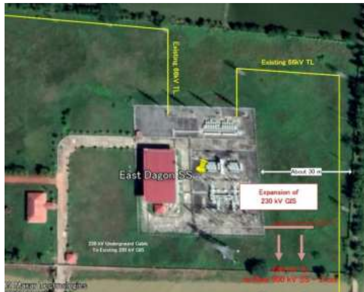
Figure 3.1-6 Location of New 230 kV Switcher at Dagon Myothit (East) Substation
