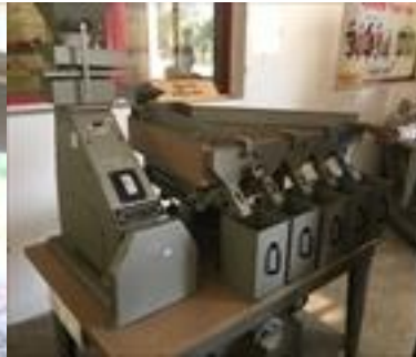
Weight grading machine (made in India)
