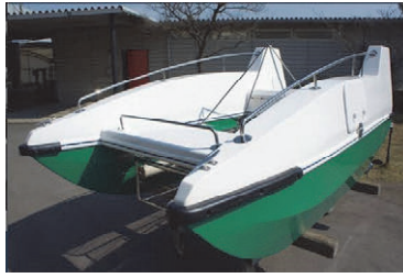
Small radio-controlled floating litter collection ship
