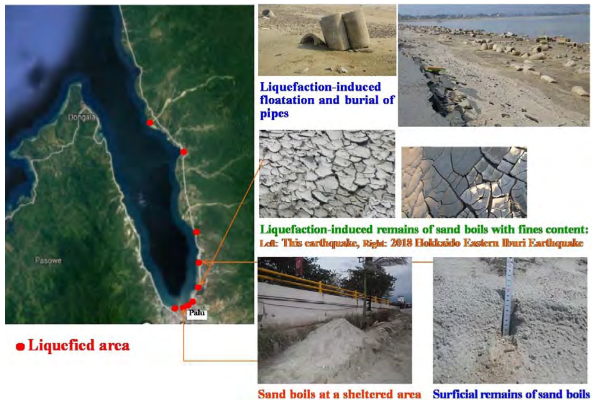
Figure 20 : Extensive Liquefaction in Coastal Areas
