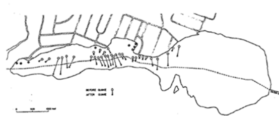
FIG. 6.—MOVEMENTS OF HOUSES IN SLIDE AREA
