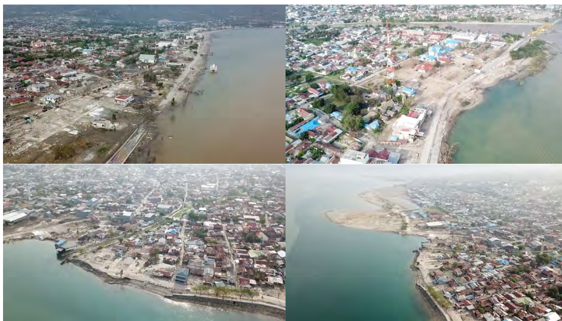
Figure 23 : Collapse by liquefaction or simple landslides occurred at many places along coastal line
