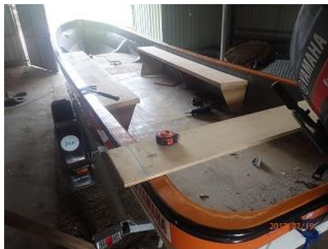
Photo 2: The project boat is under renovation for installing deck board (Tahira).
