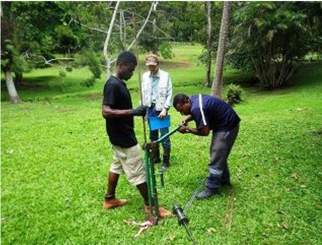
Photo 1: Mr. Imai of JICA, supervising the work of soil survey at the proposed site for Information Center (VNP).
