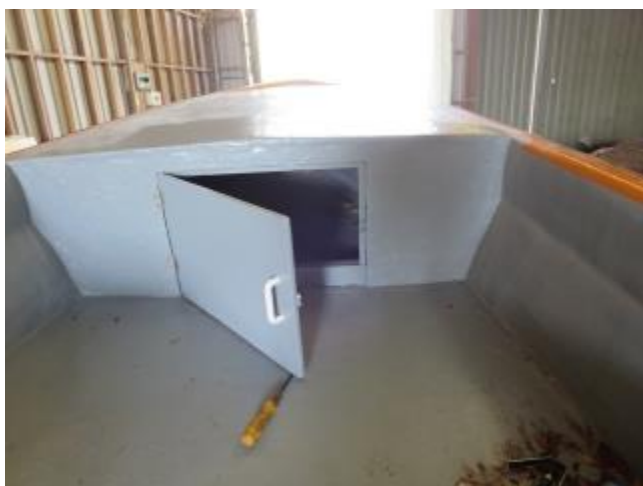
Photo 9: Front container was installed to the project dinghy, which assists project activity to be more efficient (Tahira).
