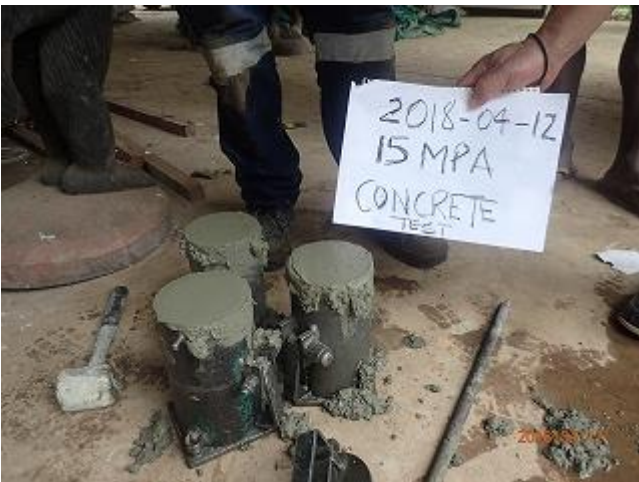
Photo 3: Workers of cement company are conducting concrete test for checking strength of concrete (VNP).
