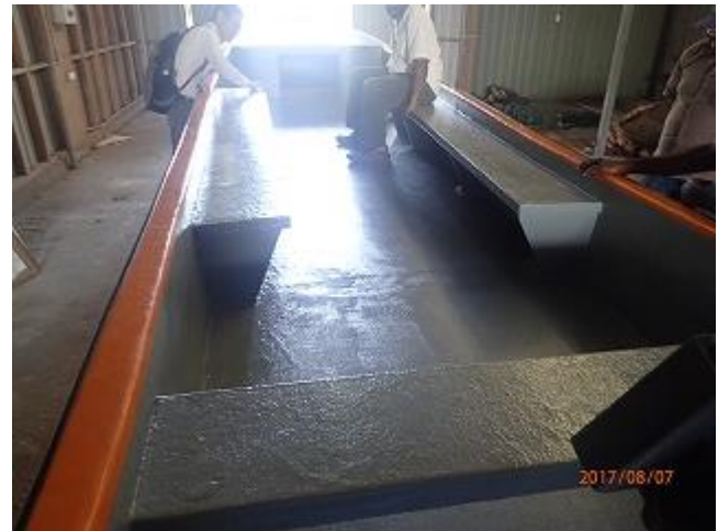
Photo 10: Installing a deck board to the project dinghy has been completed (Tahira).
