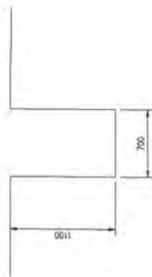
110 mm UPVC EXCAVATION SECTION SCALE 1:25
