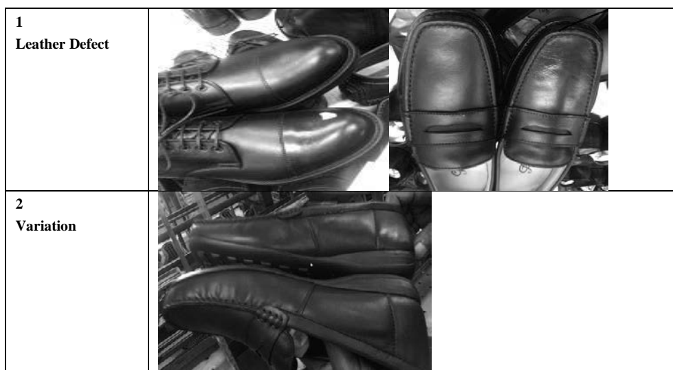
Photo-1 Poor leather (top) and bad color (bottom)
