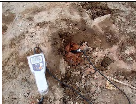
2. Fumarole with maximum temperature 99.1 °C in Asedemu area. Gas sample was collected in MP study. Dry steam is dominated.
