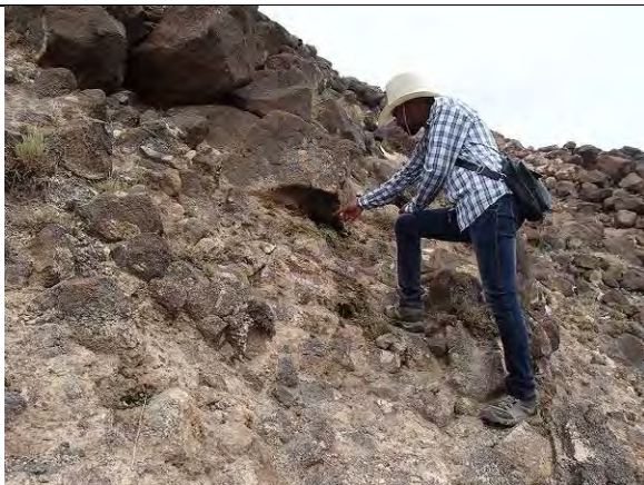
11. Fumaroles along fault F3 with maximum temperature 60.7 °C. Dry steam is dominated.
