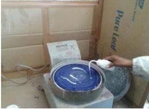
Fig.3 Maquina com DP a 3µm
